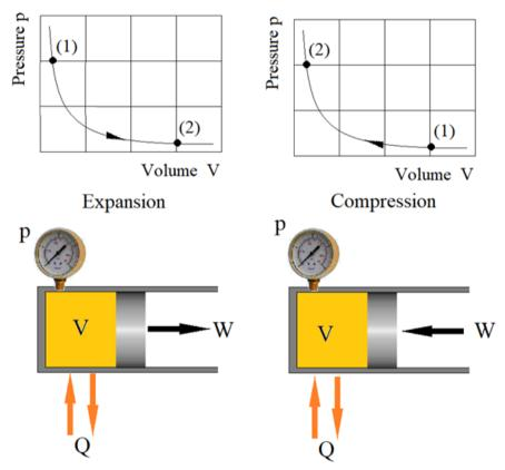
Depending on whether the fluid is heated or cooled as it is expanded or compressed, a family of such curves is obtained as shown next. It has been discovered that these curves follows the mathematical law
