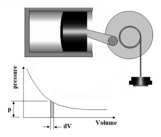
Assume that there is no pressure outside. If the string holding the weight was cut, the gas pressure would slam the piston back and the energy would be dissipated first by acceleration of the moving parts and eventually as friction. The expansion would be unresisted.
