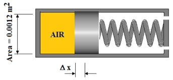
a. The spring force is directly proportional to movement such that  $\Delta F/\Delta x = k$
