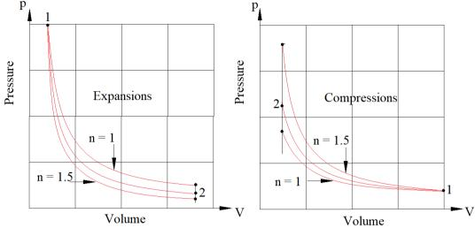
The following derivation is not strictly needed at this level but you would do well to study it. We will start by studying the expansion of a fluid inside a cylinder against a piston which may do work against the surroundings.
