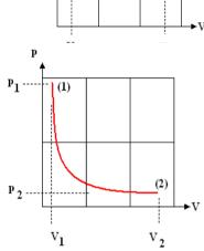
A gas is compressed from 1 bar and 100 cm<sup>3</sup> to 20 cm<sup>3</sup> by the law  $pV^{1.3} = constant$ . Calculate the final pressure.
