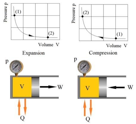
Depending on whether the fluid is heated or cooled as it is expanded or compressed, a family of such curves is obtained as shown next. It has been discovered that these curves follows the mathematical law
