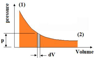
If the expansion is carried out in equilibrium, the force of the fluid must be equal to the external force F. It follows that F = p A
