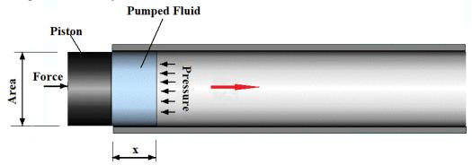
The fluid pressure is  $p N/m^2$ . The force needed on the piston is: F = pA
