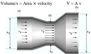
The mass flow rate is obtained by multiplying the volume by density so  $\mathbf{m} = \rho \mathbf{A} \mathbf{v}$
