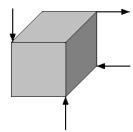
**Non - concurrent coplanar** means that the force act in different lines but only on one plane, in other words two dimensions only. There will be a resultant force and a resultant moment of force but only in the plane of the paper.
