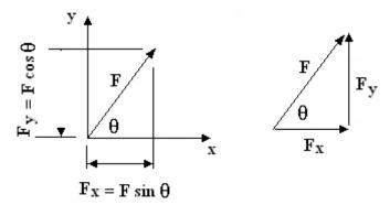
The vertical component of F is called  $F_y$  and may be found from trigonometry as  $F_y = F \sin \theta$
