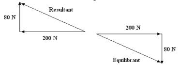
The force needed to keep the body in equilibrium must be equal and opposite of the resultant. In other words the body needs 80 N down to cancel the 80 N up and 200 N to the right to balance the 200 N to the left.
