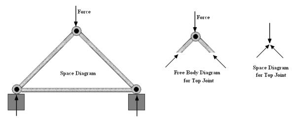
When we draw a diagram to enable us to add or subtract vectors, it is called a *Vector Diagram* as shown in the following examples.
