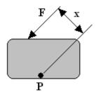
In order to demonstrate the effect of the moment arm, try suspending a kg mass from a stick and hold it out horizontally. If the mass is suspended from the far end of the stick, it is very difficult to hold up. If the mass is suspended from the end close to the hand, it is easy to hold up. The weight is the same in both cases but the larger the moment, the harder it is to hold it up.
