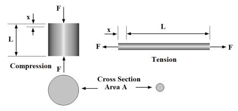
Tensile and compressive forces are called *Direct Forces*.
