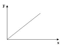
The stiffness is different for different materials and different sizes of the material. We may eliminate the size by using stress and strain instead of force and deformation as follows.
