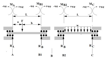
In this example the moment must be hogging at all the ends. These are the ones we use in the calculations so the fixing moments are -M on the left and +M on the right of each section.
