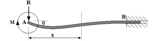
The left end must not deflect so a force R must be applied also. The bending moment any distance x from the end is
