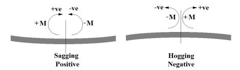
Sagging is positive and hogging is negative. At any point on the beam the bending is produced by equal and opposite moments M. Clockwise is positive and anticlockwise is negative. A sagging bending moment hence consists of +M on the left of the section and -M on the right. A hogging moment is -M on the left and +M on the right.
