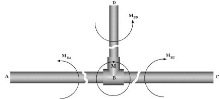
The diagram shows three members AB, DB and CB rigidly joined at B. When a moment M is applied at B the joint will twist an angler  $\theta$ . The stiffness of each member as seen from B is
