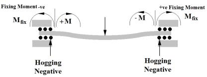
The beam is hogging at both ends. The fixing moment is the moment counteracting the bending moment in the beam. This is negative on the left end and positive on the right end. This will be used in the following examples.
