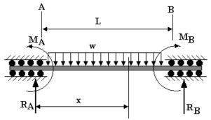
In this case the reactions are  $R_A = R_B = wL/2$ The bending moment at distance x from the left end is
