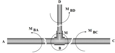
The moment M applied at the joint is distributed to the members in a proportion that depends on the stiffness of the member as seen from the joint. The moment at B is distributed to each member as shown.
