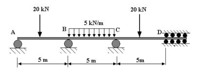
Calculate Fixing Moments and Stiffness Factors For B.
