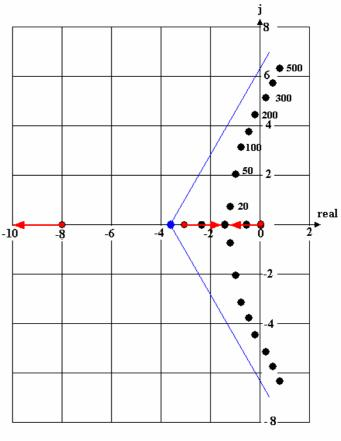
We are finding the roots of  $s^3 + 11s^2 + 24s^1 + ks^0$ . If a calculator that solves roots is available then the roots can be solved for various values of k and a precise plot obtained as shown.
