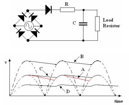
Graph A shows a typical full wave rectified voltage. During the time the voltage is rising, the capacitor charges and when the voltage starts to fall, the capacitor discharges. The result is DC plus an AC ripple.
