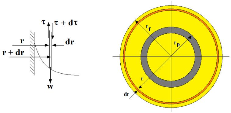
Consider an elementary thin cylindrical layer that makes an element of flowing down the outside of the pipe. The length is δx, the inside radius is r and the radial thickness is dr. The weight of the element is w and the shear stress on the surface increases by dτ from the inner to the outer surface. The velocity at any point is v and the dynamic viscosity is μ.
