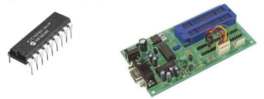
The development module needs a computer to run programming software, such as Circuit Wizard. The computer will connect through a serial port or a USB port. When the program has been simulated and works as required, it is downloaded to the PIC microcontroller. The controller does not need the computer afterwards as it works independently. For mass produced machines the chips are all programmed and then embedded in the system.
