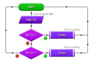
**GENIE Traffic Lights**—This flowchart determines the behaviour of the microcontroller.
