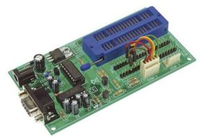
The development module needs a computer to run programming software, such as Circuit Wizard. The computer will connect through a serial port or a USB port. When the program has been simulated and works as required, it is downloaded to the PIC microcontroller. The controller does not need the computer afterwards as it works independently. For mass produced machines the chips are all programmed and then embedded in the system.
