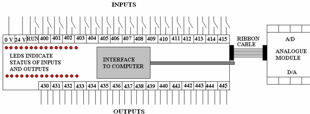
All the communication with the PLC is digital whether we are talking about the A/D module above using the ribbon cable or the communication with computers and networks using various types of mediums. The digital information has to be in a standard form.
