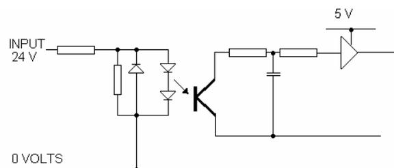
They have the advantage of reducing the effects of spurious pulses generated from electro magnetic sources. It is also a safety feature to prevent live voltages appearing on the input lines in the event of a fault.
