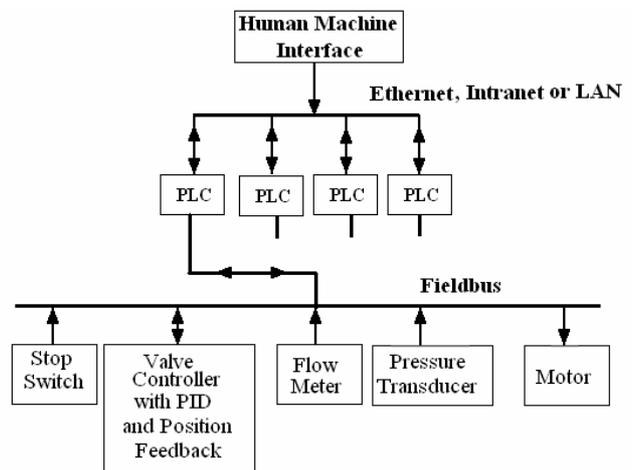
The HMI at the top is the **MASTER** and the plcs are the **SLAVES**. Communication between them is master to slave or slave to master. Communication between the PLCs is peer to peer. There are various protocols and standards laying down the way they communicate such as:
