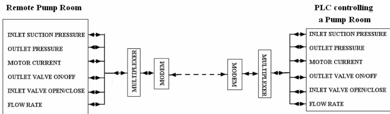
The multiplexer and modems must be able to tell when to send and when to receive, what channel is being used and be able to handle the type of digital signal in use. To do this we must have standards of **PROTOCOL**. Protocol is essential for any digital system to communicate with another.
