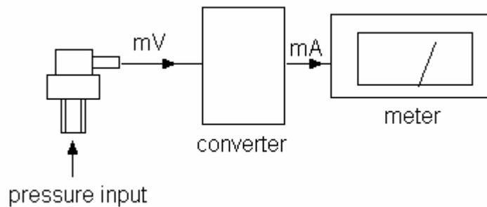
The system consists of pressure transducer connected to a converter. The output mV is related to the input pressure by  $V = 30 p$  where p is in bar and V is in mV. The converter output in mA is related to the input by  $I = 4 + 0.2V$ . The current is sent to a meter. What is the pressure when the meter indicates 15mA? (1.833 bar)
