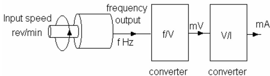
The tachometer produces one cycle of electricity for every revolution. The f/V converter converts the frequency into mV such that a  $V = 0.6 f$ . The V/I converter produces an output of 0.8 mA/mV. Calculate the output when the tachometer is turned at 3000 rev/min. (24 mA)
