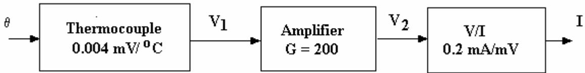
Determine the current when the temperature is 120°C. (19.2 mA)
