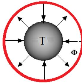
A is the envelope area of the enclosed body. For difficult shapes like that shown below, it should be regarded as the area that would be obtained by stretching an elastic membrane over it.
