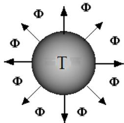
A hot body radiates energy in the form of electromagnetic radiation. It is found that the energy radiated depends upon the absolute temperature to the power of 4.
