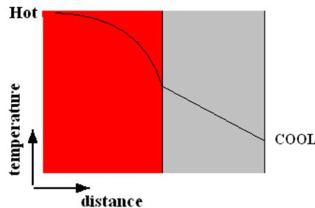
Consider a hot fluid flowing through a long pipe with heat transfer required into the wall of the pipe. The fluid in contact with the surface will reach the same temperature as the pipe at some point and further contact will not increase the transfer. The heat transfer will decrease with distance as shown. To improve the heat transfer, it is necessary to promote turbulent flow so that the fluid in the core is moved to the edges and comes in contact with the wall.
