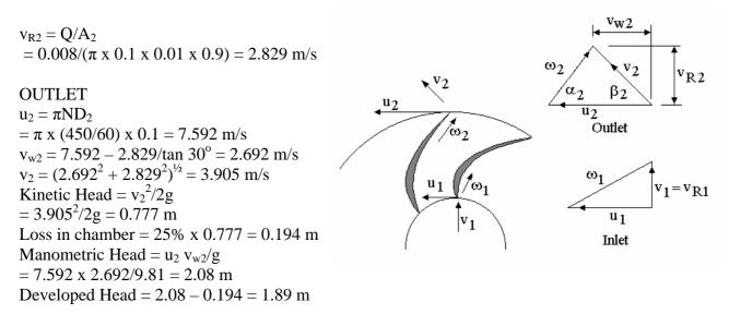
$\Delta h = u_2 v_{w2}/g = (u_2 - Q/A_2 \tan \alpha_2)$ When there is no flow Q = 0 so  $\Delta h = u_2 v_{w2}/g - u_2 = (7.592/9.81) \times 7.592 = 5.875 m$
