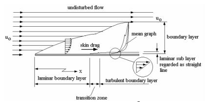
Limitations are that the flow must be turbulent with  $R_e > 10^7$  and the velocity gradient must be the same at the junction between the laminar sub layer and the turbulent level.
