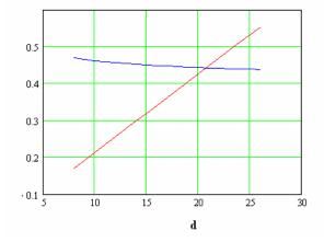
$\text{Re} = \rho u d/\mu = 998 \text{ x } 0.5 \text{ x } 0.00595/0.89 \text{ x } 10^{-3} = 3336$  $C_D = 21.389 \frac{d}{u^2} = 0.509$  $C_{\rm D} = \frac{24}{3336} + \frac{6}{1 + \sqrt{3336}} + 0.4 = 0.509$
