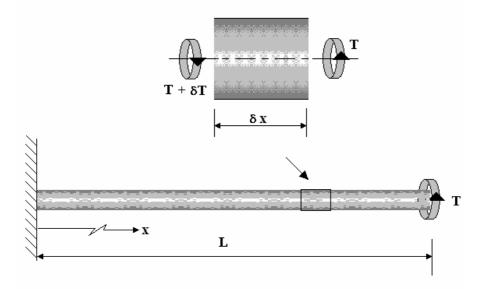
Consider an element of the shaft length  $\delta x$ . The torque at one end is slightly larger than the torque at the other by  $\delta T$ . Suppose the torque decreases uniformly with x as  $\frac{dT}{dx}$
