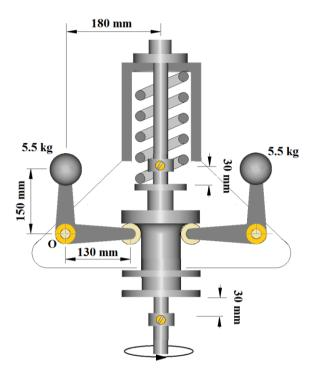
The stops are  $\pm$  30 mm from the position shown. The speed is to be set to obtain 250 rev/min and 265 rev/min at the lower and upper stops respectively.
