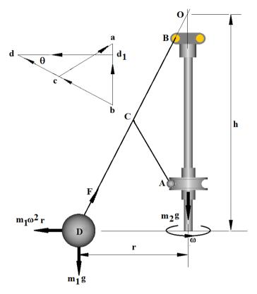
The velocity diagram is shown for the linkage and indicates the direction and relative movement of all the points. Except for the sliding sleeve these can only be at 90° to the links. Let the sleeve be sliding upwards so the movement of A relative to B can only be vertical.
