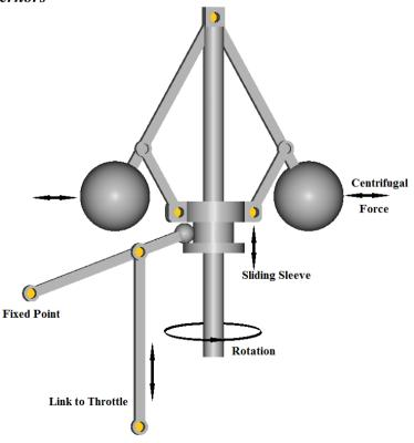
Internal combustion engines have long been used for stationary applications such as driving air compressors, pumps, electric generators and so on. The speed of the engine needs to be constant and so a governor is needed to adjust the controls according to the output speed. The same applies to external combustion engines such as gas turbines and steam turbines. The control action basically is that of adjusting a throttle of some kind that varies the flow of fuel, air or steam.
