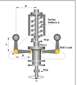
2. The same governor as Q1 has a spring rate of 40 N/mm and the initial compression is 10 mm. Calculate the speeds at the upper and lower stops.
