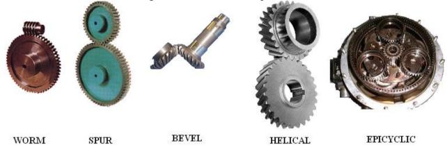
Gears are wheels which mesh with each other through interlocking teeth. Rotation of one wheel produces rotation of the other with no slip between them. The shape of the gear teeth is important in order to produce a smooth transfer of the motion.
