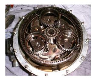
This design can produce large gear ratios in a small space and are used on a wide range of applications from marine gear boxes to electric screwdrivers.
