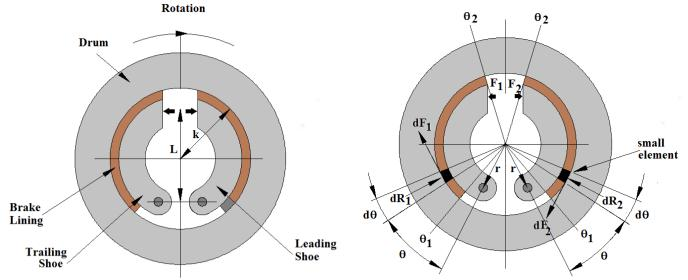
Consider a small element of the lining shaded in black. Suffix 1 indicates the trailing edge and suffix 2 the leading edge. The normal reaction force between the friction lining and the drum is dR The friction force between them is  $dF = \mu dR$
