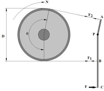
A typical band brake is illustrated. Basically these are belts rubbing on wheel. It was shown in tutorial 2 that the force in each end of the belt is related by the formula:
