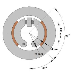
$\begin{array}{ll} F_1 = F_2 = 250 \ N & L = 150 \ mm & w = 45 \ mm \\ k = 90 \ mm & r = 75 \ mm & \theta_1 = 45^\circ = \pi/4 \ radian \\ \theta_2 = 135^\circ = 3\pi/4 & \mu = 0.45 \end{array}$
