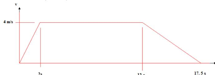
$$\text{Distance} = \text{Area under graph} = (4 \times 2)/2 + (10 \times 4) + (4 \times 5.5)/2 = 55 \text{ m}$$
