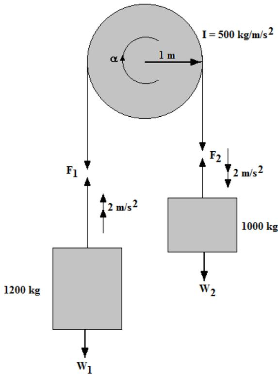
The key to this solution is to bear in mind that the acceleration of the two masses is always opposite in direction
