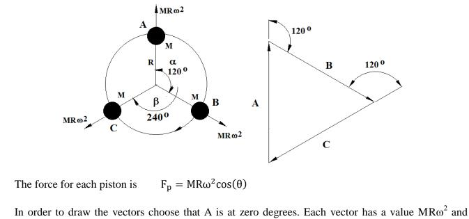
In order to draw the vectors choose that A is at zero degrees. Each vector has a value MR $\omega^2$  and adding them we see there is no resultant so there is no resultant vertical component (MR $\omega^2 \cos\theta$ ) either and so  $F_p = 0$  and this will be true whatever the crank angle.
