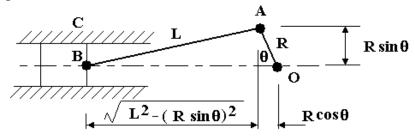
When  $\theta = 0$  the piston will be furthest left at a distance of L+R from point O. Take this as the reference point and measure displacement x from there. Remember that  $\theta = \omega t$  and  $\omega = 2\pi x N$ . The displacement is then
