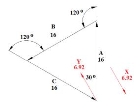
The closing vector is equal and opposite of Y 0.04Mx =  $6.92 \times 10^{-3}$  at  $30^{\circ}$  as shown.
