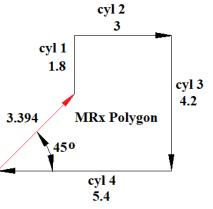
The balancing MRx on plane B is  $\sqrt{\{(2.4 \times 10^{-3})^2 + (2.4^2 \times 10^{-3})\}} = 3.394 \times 10^{-3} \text{ kg m}^2$  at 45° as shown.
