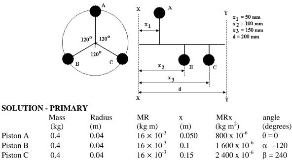
Drawing the MR polygon with A vertical we see the resultant force is zero as expected.
