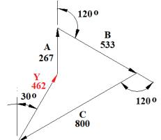
From the MRx/n polygon we get a closing vector  $Y = 462 \times 10^{-6} \text{ kg m}^2$  at 30° as shown.
