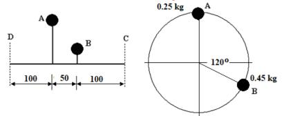
2. A compressor has three inline pistons A, B and C positioned as shown with crank radii of 80 mm and connecting rods 240 mm long. The compressor is to be balanced for primary and secondary components by placing two sets of contra rotating masses at 50 mm radius at each bearing, one running at the crank speed for the primary balance and one at double the speed for secondary balance. Determine the masses and angles relative to crank A.
