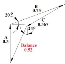
Using trigonometry or scaling from the diagram reveals that for balance we need 0.52 R so  $M_D = 0.52$  kg at the same radius and it must be placed at 204° to crank A at located at D.
