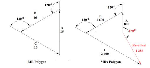
Draw the MRx polygon and by scaling or calculation the resultant is  $1 \ 386 \times 10^{-6} \text{ kg m}^2$ The resulting moment about plane XX is  $M_x = \omega^2 \times 1 \ 386 \times 10^{-6} \cos 30^\circ$  $M_x = 30^2 \times 1 \ 386 \times 10^{-6} \cos 30^\circ = 1.08 \text{ Nm}$
