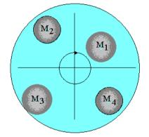
The result obtained would be the same whatever the value of  $\omega$  and when  $\omega = 0$  we have static balance. In order to make the solution easier, we may make  $\omega = 1$  and calculate M r for each vector. This is called the M r polygon or vector diagram.
