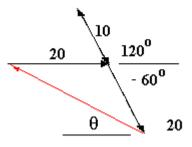
The red vector produces balance and may be calculated or measured. The length is 26.5 g m and the angle  $\theta$  is 19.1°. This is placed on plane A. The table may be further completed.
