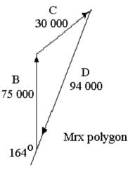
Scaling the vector D which closes the triangle we find Mrx for D = 94 000 = 22 500 M<sub>D</sub> Hence M<sub>D</sub> = 94 000/22 500 = 4.17 kg and it is positioned 2540
