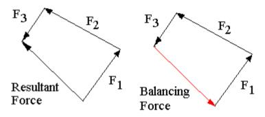
If the system was balanced, there would be no resultant force so the force needed to balance the system must be equal and opposite of the resultant (the vector that closes the polygon). The balancing mass  $M_4$  is then added at a suitable radius and angle such that the product M r is correct.
