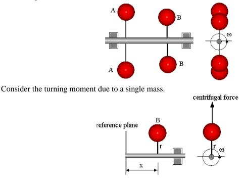
The centrifugal force produced is  $F = Mr\omega^2$
