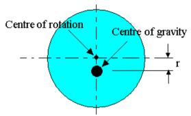
If the centre of gravity is distance r from the centre of rotation then when it spins at  $\omega$  rad/s, centrifugal force is produced. This has a formula C.F.= M  $\omega^2$  r where M is the mass of the disc. This is the out of balance force. In order to cancel it out an equal and opposite force is needed. This is simply done by adding a mass M<sub>2</sub> at a radius r<sub>2</sub> as shown. The two forces must have the same magnitudes.
