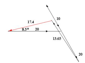
A static imbalance of 17.4 g m at 188.5° now exists and this will be countered by a force in the bearing at O. Centrifugal force =  $m\omega^2 R$  so the force on the bearing is
