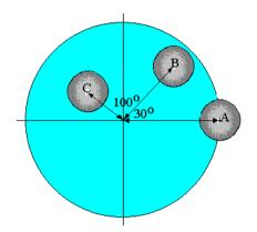
Each vector has a component in the x direction given by Mr  $\cos\theta$  and in the y direction it is MRsin $\theta$
