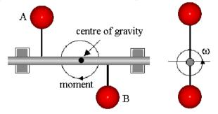
For static balance  $M_A r_A = M_B r_B$
