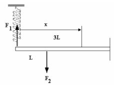
(a) The forces acting on a statically indeterminate beam cannot be resolved without some additional information. An example of this is a propped cantilever. The moments cannot be solved unless the deflection at the prop is known. In the case below, we must know the spring rate in order to relate the force to the deflection. The reactions cannot be found until the deflection has been found. When this is done, the forces may be resolved to find the reactions.
