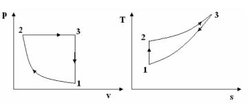
$$\eta = 1 - \frac{mc_v(T_3 - T_1)}{mc_p(T_3 - T_2)} = 1 - \frac{c_v(T_3 - T_1)}{c_p(T_3 - T_2)} = 1 - \frac{(T_3 - T_1)}{\gamma(T_3 - T_2)} \quad \text{noting } c_p/c_v = \gamma \qquad \eta = 1 - \frac{\left(1 - \frac{I_1}{T_3}\right)}{\gamma\left(1 - \frac{T_2}{T_3}\right)}$$
